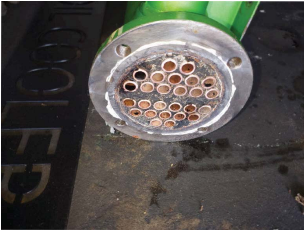
OIL COOLER BEFORE CLEANING
