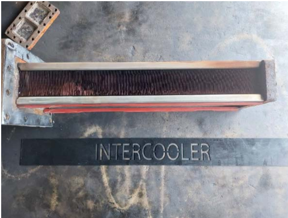
INTERCOOLER BEFORE CLEANING
