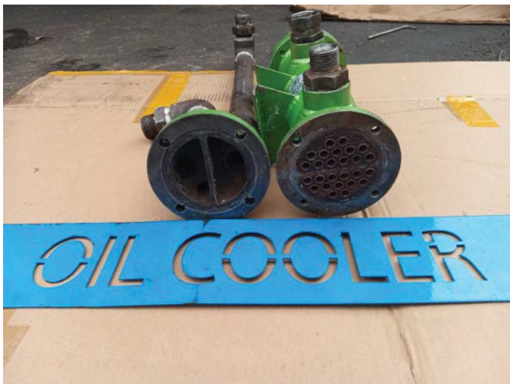
OIL COOLER AFTER CLEANING
