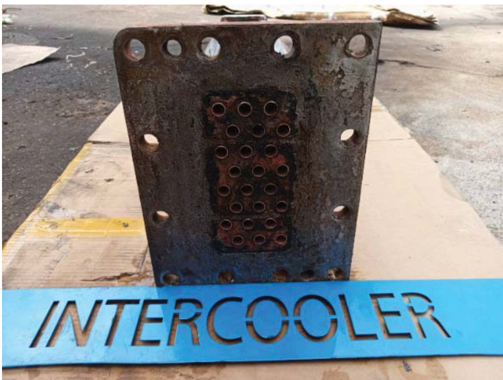
INTERCOOLER AFTER CLEANING
