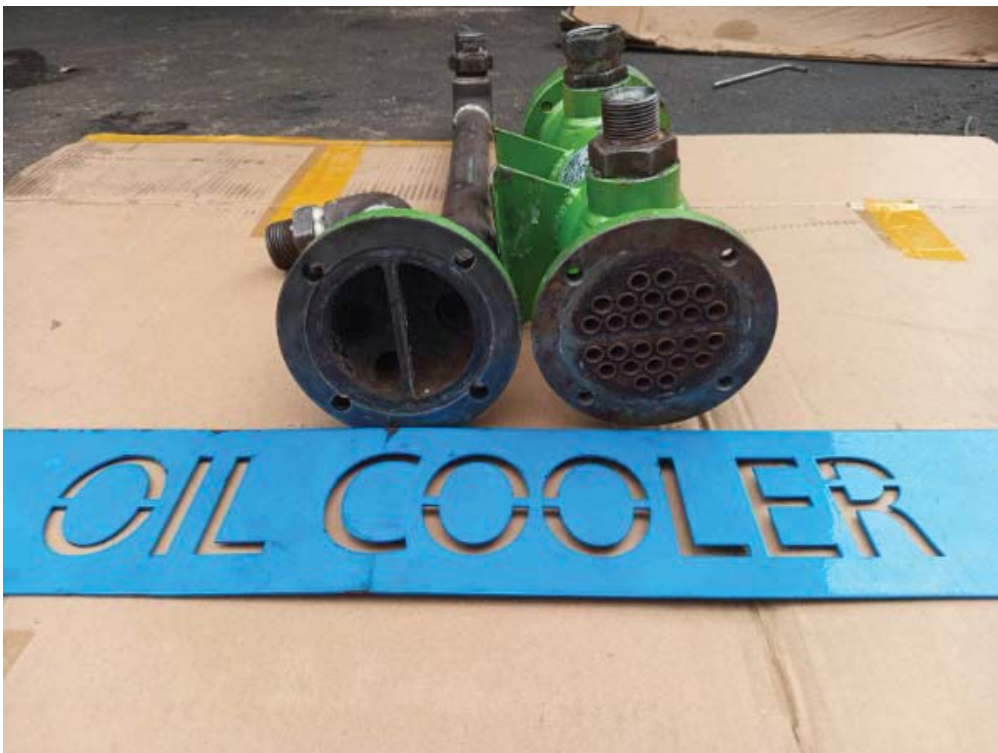
OIL COOLER AFTER CLEANING
