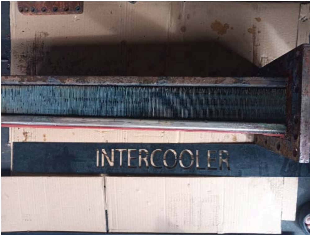
INTERCOOLER BEFORE CLEANING
