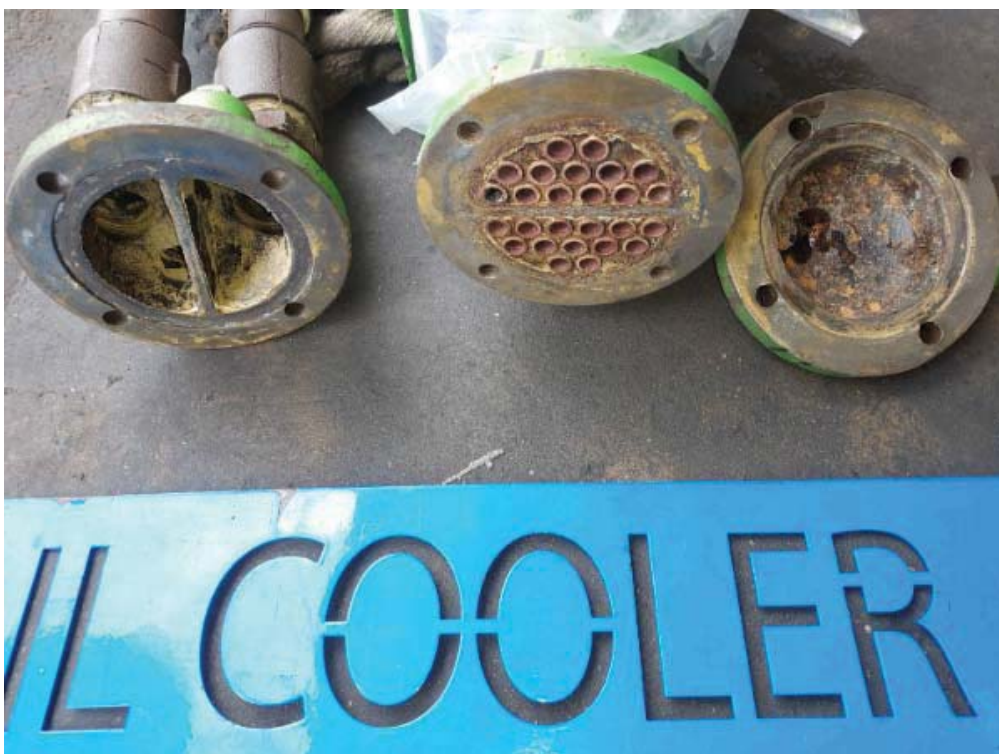
OIL COOLER AFTER CLEANING
