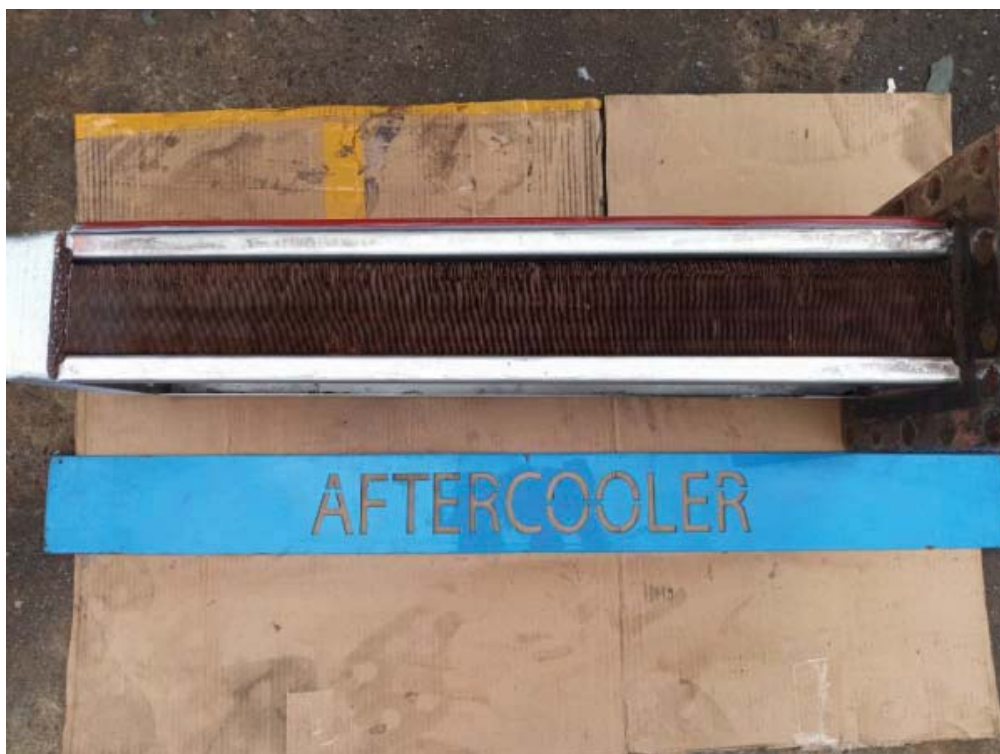
AFTERCOOLER AFTER CLEANING
